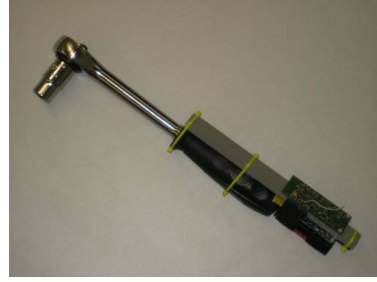
Fig. 3. Left: worker mounting the front door of the car. Right: socket wrench equipped with acceleration sensing wireless nodes.
