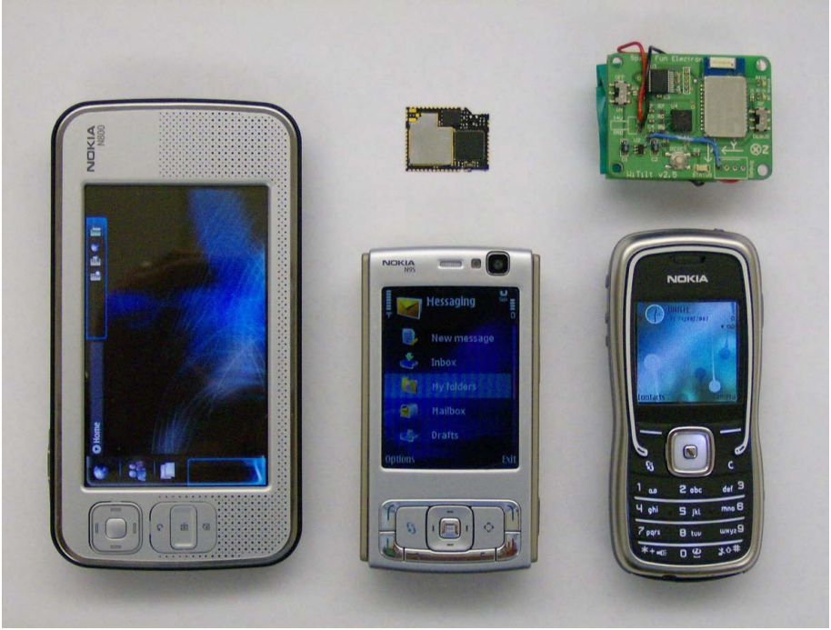
Fig. 4. Mobile devices currently integrated into the CenceMe system: the Nokia N800 Internet Tablet, Nokia N95, Nokia 5500 Sport, Moteiv Tmote Mini (above the N95), and prototype BlueCel accessory (above the 5500)
