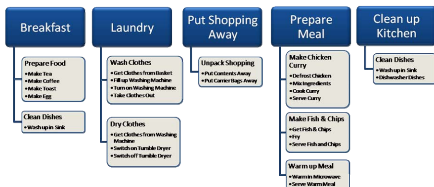
Fig. 7. The root plan is the ADL (e.g. Breakfast), the child nodes are the sub-plans/activities which are made up of tasks which are also known as single step plans
