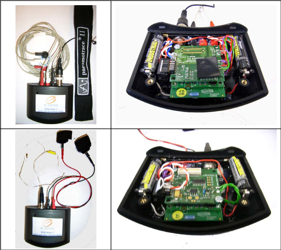
Fig. 2. BSN components: The figure shows outside and inside view of the developed BSN nodes for ECG/breathing node (above) and EDA/skin temperature node (below)
